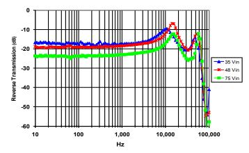
Figure 21: Magnitude of incremental reverse transmission (RT = in/iout) for minimum, nominal, and maximum input voltage at full rated power.
