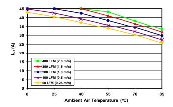
Figure 5: Maximum output power derating curves vs. ambient air temperature for airflow rates of 50 LFM through 400 LFM with air flowing from input to output (nominal input voltage).
