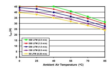
Figure 7: Maximum output power derating curves vs. ambient air temperature for airflow rates of 50 LFM through 400 LFM with air flowing from output to input (nominal input voltage).
