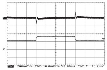
Figure 11: Output voltage response to step-change in load current (50%-75%-50% of lout(max);  $dI/dt = 0.1A/\mu s$ ). Load cap:  $15\mu F$ , 450mOhm ERS tantalum cap and  $1\mu F$  ceramic cap. Top trace: Vout (200mV/div). Bottom trace: lout (20A/ div).
