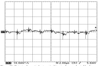
Figure 16: Output voltage ripple at nominal input voltage and rated load current (10 mV/div). Load capacitance:  $1\mu$ F ceramic capacitor and one  $15\mu$ F tantalum capacitor. Bandwidth: 20 MHz. (See Figure 13).
