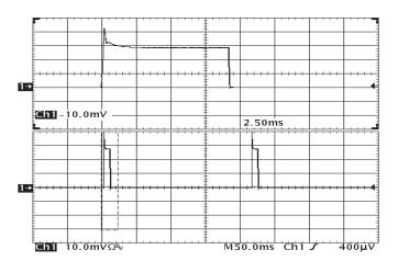
Figure 18: Load current (20*A*/div) as a function of time when the converter attempts to turn on into a 1 m $\Omega$  short circuit. Top trace (2.5ms/div) is an expansion of the on-time portion of the bottom trace.
