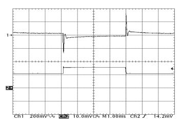
Figure 12: Output voltage response to step-change in load current (50%-75%-50% of Iout(max):  $dI/dt = 5A/\mu$ s). Load cap:  $470\mu$ F, 15mOhm ESR tantalum cap and  $1\mu$ F ceramic cap. Top trace: Vout (200mV/div). Bottom trace: Iout (20A/div).
